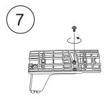
7) Make sure the angle adjustment is straight, then remove center screw
