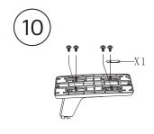
10) Pick any of the screw holes to install Bracket B and use the same screw to secure it
