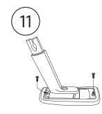
11) Reinstall the arm pad using the same two screws and secure the pad.
