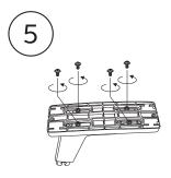
5) Remove four screws that secure the part for sliding
