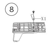
8) Place Bracket A and use the same screw to secure it
