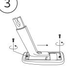
3) Slide the arm pad forward and remove screws
