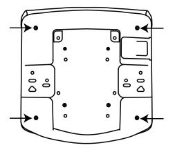
4) Re-attach the seat pan to the slip cover using the four screws from step 1
