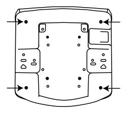
1) Remove 4 screws outermost four corners to separate seat pan slip cover
